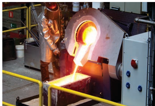
Byproducts processing facilities – Smelting furnaces 350 kg induction furnace dedicated to the recycling of solid residues in metallic bath
