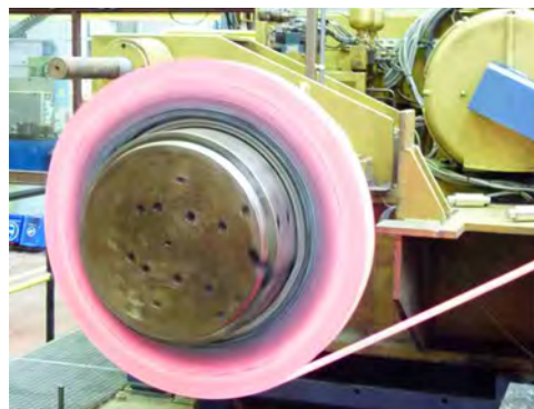
Hot rolling pilot mill available at CRM Gent in collaboration with OCAS (MPC joint-venture)
