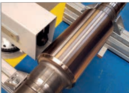
Photo 2: Pilot rolls electro-plated with a new developed coating to substitute CrVI-plating
