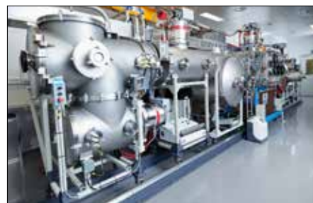
Roll-to-Roll pilot line for upscaling the stainless steel bipolar plate coating for fuel cells
