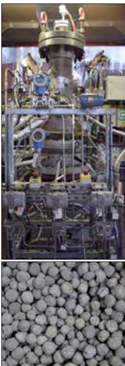
HUGE Thermo-conversion pilot facility in 'Direct Reduction' configuration and DRI produced in the HUGE reactor
