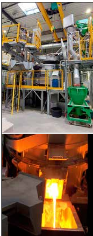
Fig. 1 – Pilot plasma furnace simulating EAF, SAF or slag valorization routes
