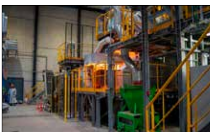
Fig. 2 - Pilot plasma furnace simulating EAF, SAF or slag valorization routes
