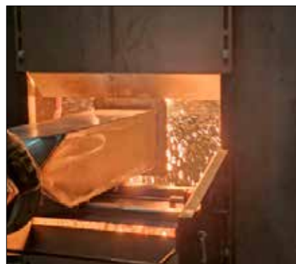
Fig. 4 - Pilot scale dry slag granulation
