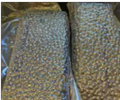
Fig. 1 - Samples (vacuum-packed) produced in CRM Group's pilot DRI reactors
