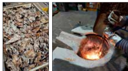
Fig. 3 - Scrap melting to assess quality improvement after scrap sorting and processing
