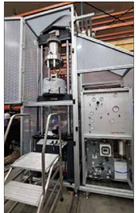
Fig. 4 – Test facilities for material behaviour under hydrogen exposure
