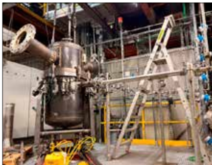
Fig. 1 – Reactor for Direct Reduction of Iron
